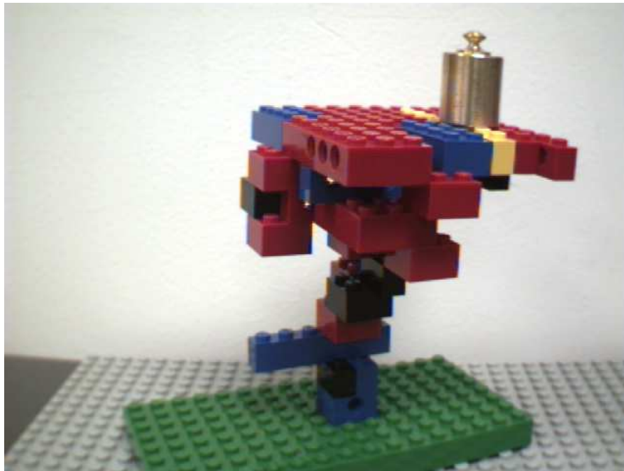
fig. 15. Lego table as specified by the diagram of fig. 4, holding a 50g weight.
